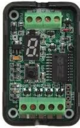
Figure 3-3: Solar Panel Light Controller Battery Charge
