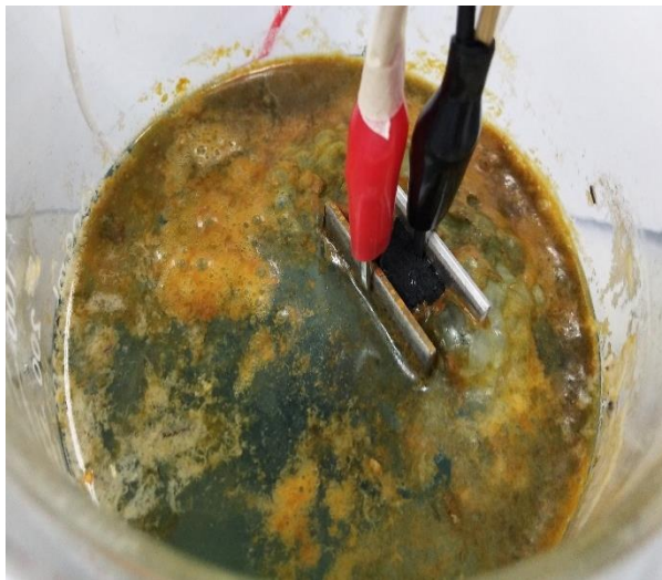
Figure 4.8 Flocculation occurred at top of the wastewater sample
