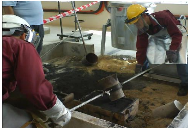
Figure 3.7: Pouring the molten metal from ladle to mould
