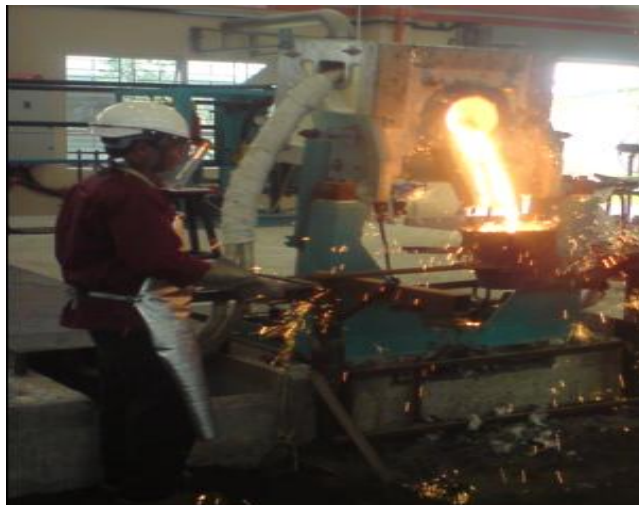
Figure 3.6: Pouring the molten metal from furnace to ladle
