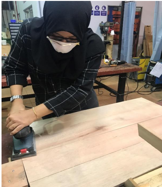
Sanding the woods using stebrates papers to get a smooth surface
