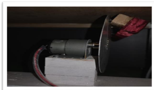
Figure 4.2 Rotating mechanism of baby cradle
