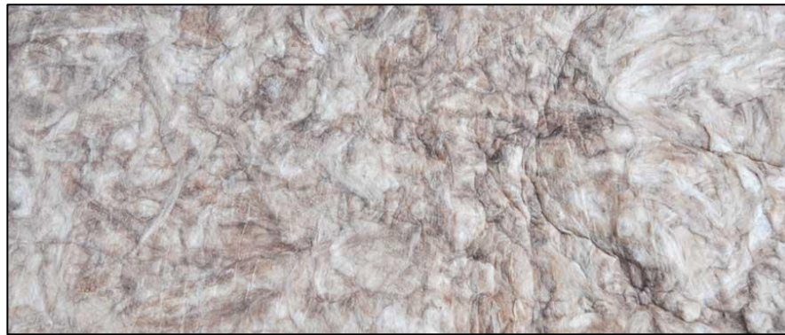
Figure 2.3: The Structure of mineral wool (GreenSpec, 2018)
