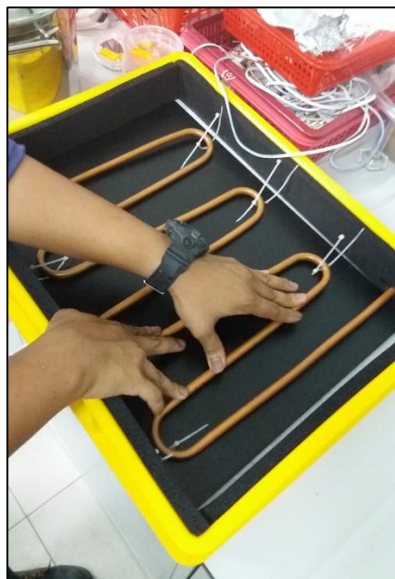
Figure 3.14: The copper were attached to the aluminum plate by using cable ties.
