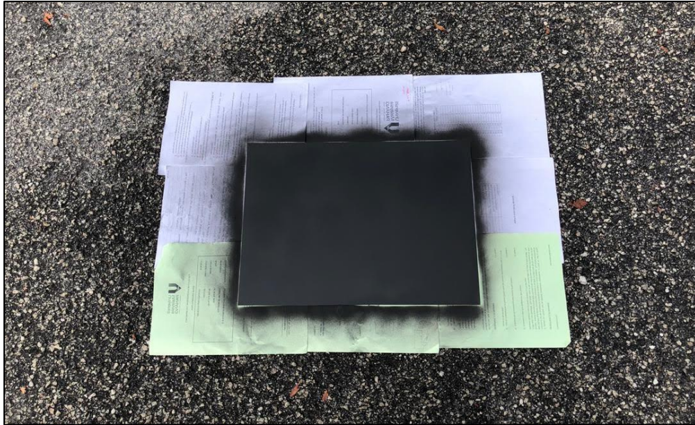
Figure 3.11: The aluminum were coated with dull black paint
