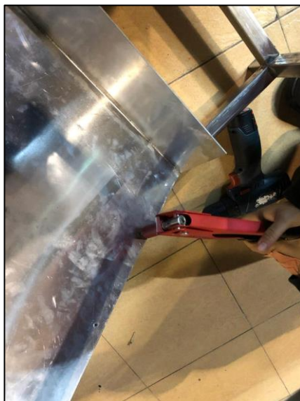
Figure 3.9: The hand riveter were used to rivet the aluminum plate to the rack
