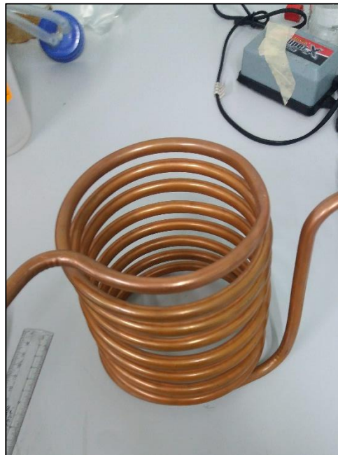
Figure 3.15: The winded copper coil ready to be installed into the tank
