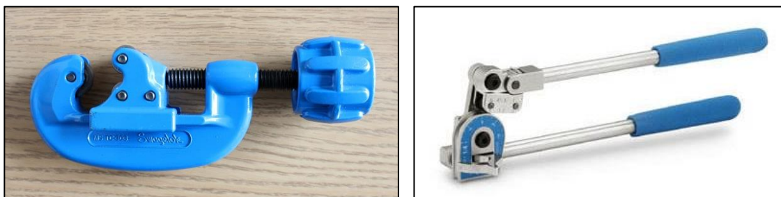
Figure 3.12 (a) and (b): The tools used to cut and bend the copper tube
