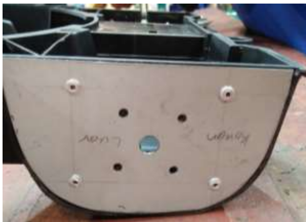
Figure 3.19 Aluminum plate attached on the trimmer's body
