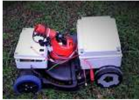
Figure 3.23 Two electrical controller box were attached on the trimmer's body
