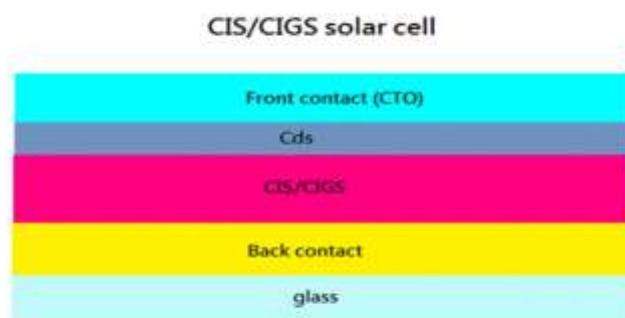
Figure 2.12 Composition of CIS/CIGS thin film
