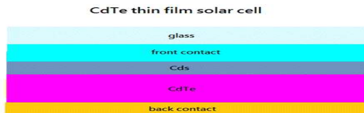
Figure 2.11 Composition of Cadmium telluride (CdTe) thin film
