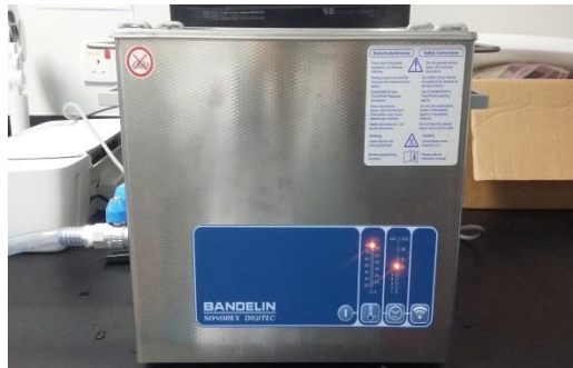
Figure 2A Bandelin Sonoren Digitec ultrasonic water bath used to extract C. asiatica
