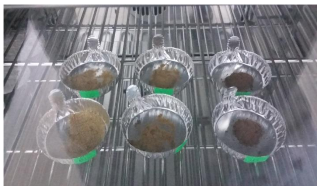
Figure 5A C. asiatica powder samples used for hygroscopicity test
