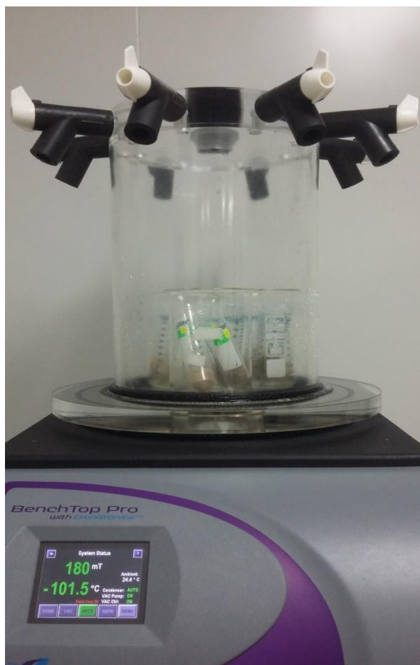
Figure 3.5 Freeze drying process via VirTis BenchTop Pro with Omnitronics-8L
