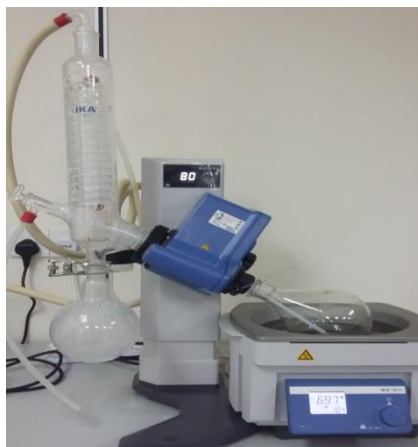
Figure 3A Rotary evaporator used to concentrate the C. asiatica extracts volume
