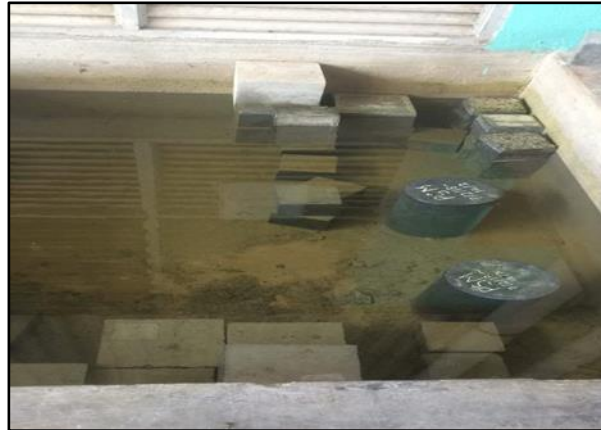
Figure 3.14 Plain UHPC and rubberized UHPC were cured in water curing tank
