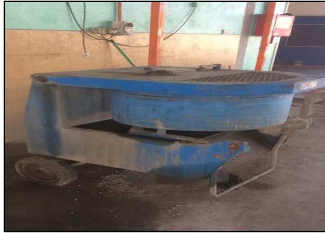
Figure 3.9 Concrete pan mixer for mixing process
