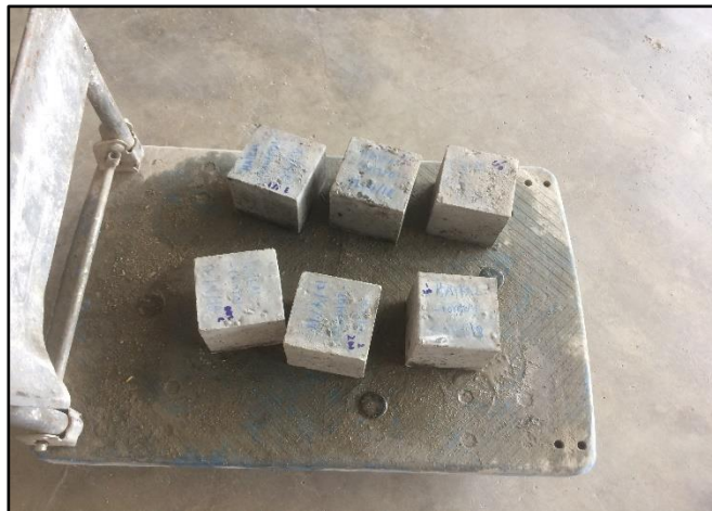
Figure 3.13 UHPC samples for weight loss test
