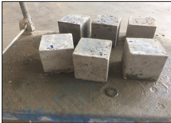
Figure 3.12 UHPC samples for compressive strength test
