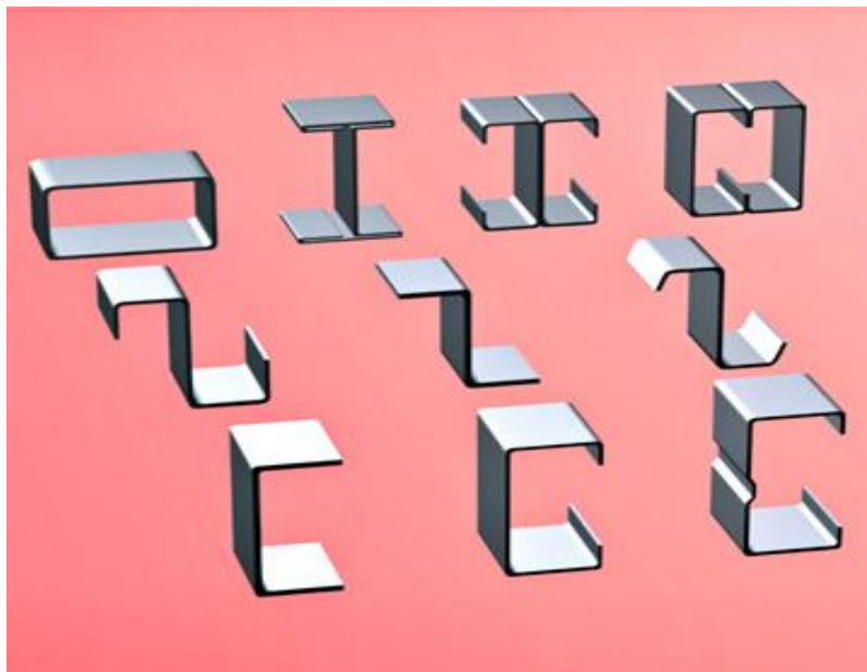
Figure 1.1 Shape of cold-formed steel
