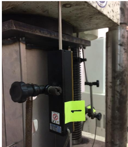
Figure 3.9 Transducers 1 for vertical displacement
