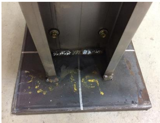
Figure 3.5 Welded connection at top and bottom
