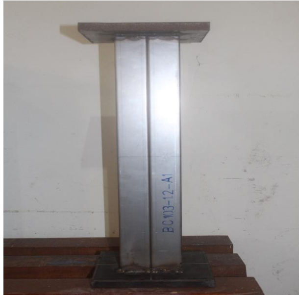
Figure 3.1 Base plate welded for top and bottom
