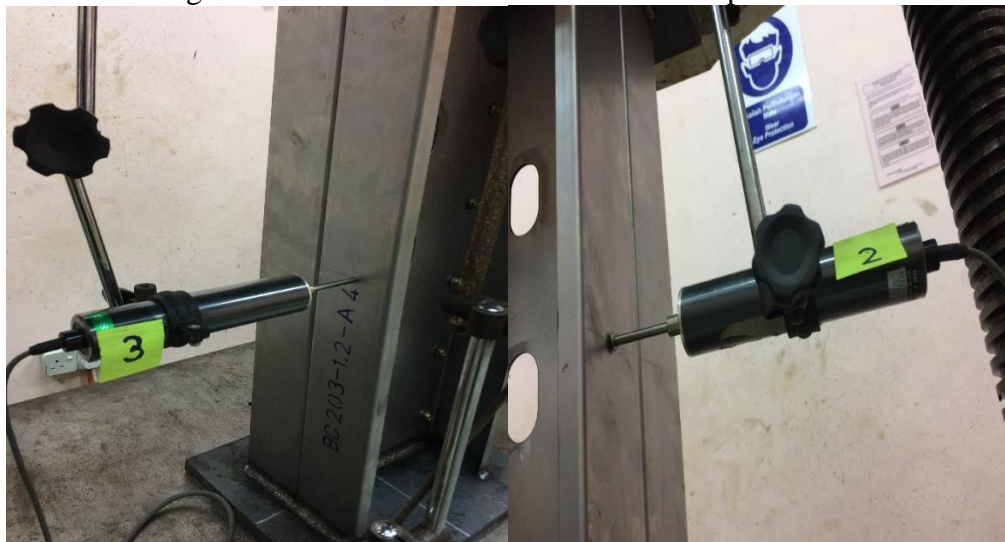
Figure 3.10 Transducers 2 and 3 for horizontal displacement
