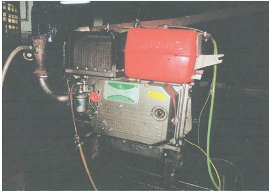
Figure 5. Test engine mounted on dynamometer bed.
