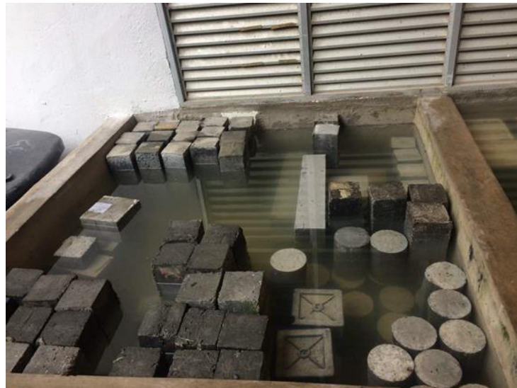
Figure 3.6 Water curing process
