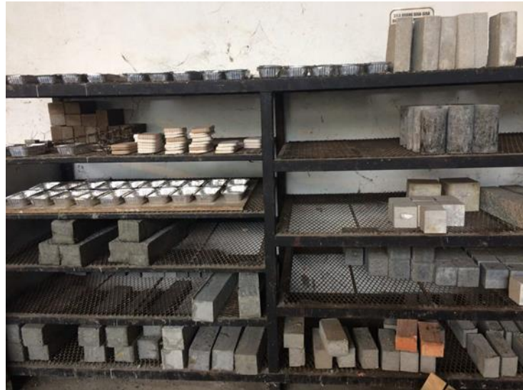
Figure 3.5 Air curing process
