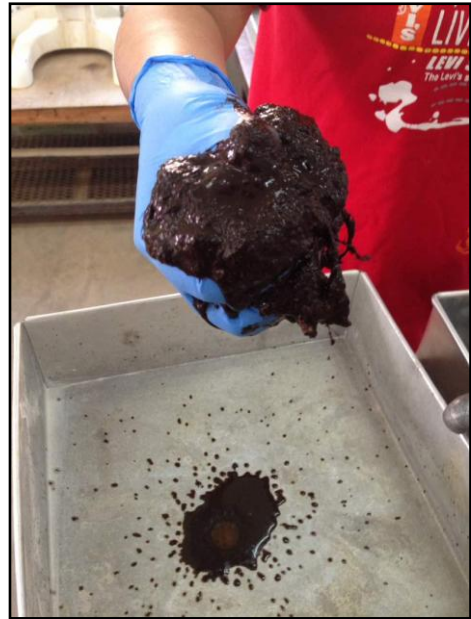
Figure 4.2: Muddy water comes out when squeezing the peat.
