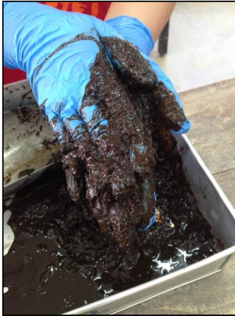
Figure 4.1: Rubbing test of Van Post Scale
