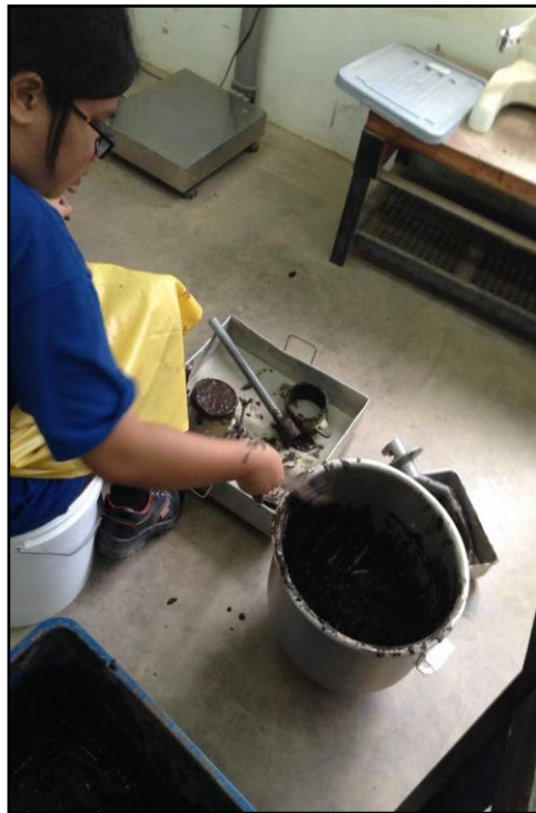
Figure 3.52: Mixing process and compacted sample
