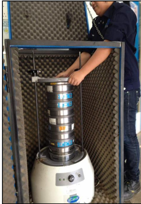
Figure 3.12: Putting the sample into sieve shaker
