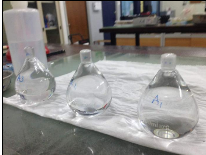
Figure 3.27: Specific gravity performed using density bottle
