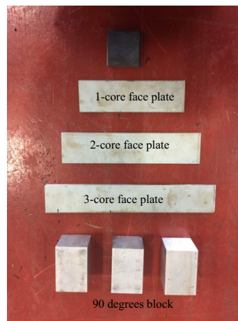
Figure 3. Face and web plates.
