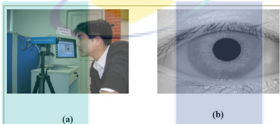
Figure 2.6 CASIA-Iris V1 (a) capturing device, (b) captured image
