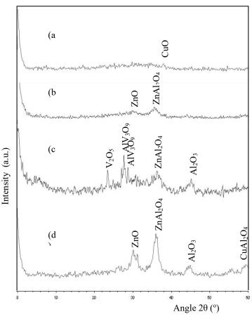
Fig. 7: XRD diffractograms of the catalyst samples (a) Cu<sub>40</sub>Zn<sub>10</sub>V<sub>10</sub>Al<sub>40</sub> oxides (b) Cu<sub>10</sub>Zn<sub>40</sub>V<sub>10</sub>Al<sub>40</sub> oxides (c) Cu<sub>10</sub>Zn<sub>10</sub>V<sub>40</sub>Al<sub>40</sub> oxides and (d) Cu<sub>20</sub>Zn<sub>20</sub>V<sub>20</sub>Al<sub>40</sub> oxides.
