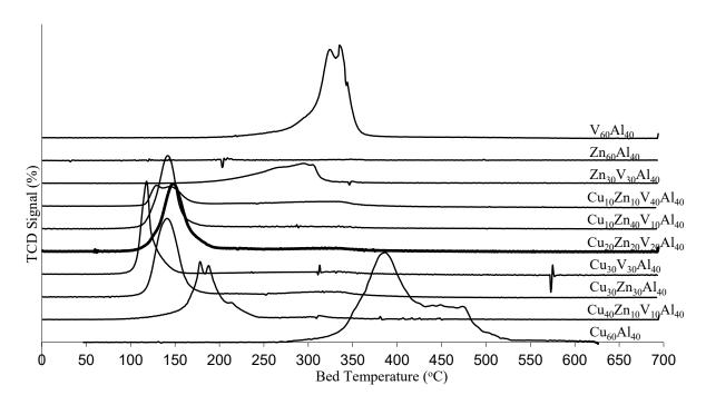
Fig. 9: TPR results for the prepared catalyst.
