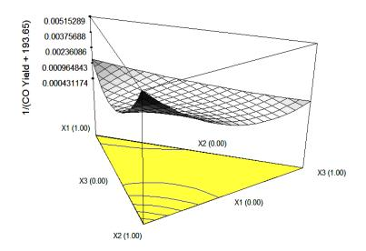
Fig. 15: Reciprocal CO yield with a constant of 193.65 as a function of catalyst metal composition, the best fitted model.
