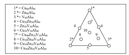
Fig. 1: Simplex Centroid Design on metal mass composition. Starred numbers denote the replicated samples.
