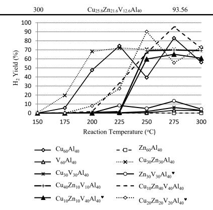
Fig. 12: Hydrogen yield versus reaction temperature at steady state for autothermal reforming of methanol. The catalyst legends added with superscript ♥ to denote having an amorphous structure.
