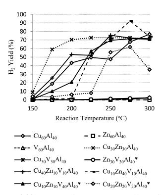
Fig. 10: Hydrogen yield versus reaction temperature at the steady state SRM process for various catalysts. The catalyst legends added with superscript ♥ to denote having an amorphous structure.
