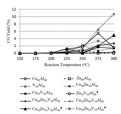
Fig. 14: CO yield as a function of reaction temperatures for various catalysts for autothermal reforming of methanol. The catalyst legends added with superscript ♥ to denote having an amorphous structure.
