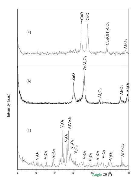
Fig. 2: XRD diffractograms of the catalyst samples (a)  $Cu_{60}Al_{40}$  oxides, (b)  $Zn_{60}Al_{40}$  oxides and (c)  $V_{60}Al_{40}$  oxides.
