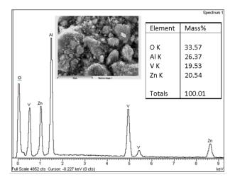
Fig. 6: Scanned image with energy dispersed X-ray confirmed that no other material appeared in the catalyst and the composition of the catalyst was approximately same as initial mixing.
