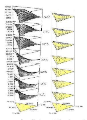
Fig. 13: Response surface of hydrogen yield against catalyst metal mass fraction of cuprum, zinc, and vanadium, X1, X2 and X3, respectively,
