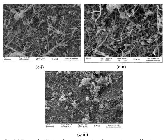
Fig. 5: Micrographs of tri-metal co-precipitated catalyst at various magnifications: (a) Cu<sub>30</sub>Zn<sub>30</sub>Al<sub>40</sub> at 10000 times, (b) Cu<sub>30</sub>V<sub>30</sub>Al<sub>40</sub> at 10000 times and (c) Zn<sub>30</sub>V<sub>30</sub>Al<sub>40</sub> at (c-i) 10000 times, (c-ii) 15000 times and (c-iii) 1000 times.
