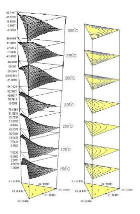
Fig. 11: Response surface of hydrogen yield against catalyst metal mass fraction of cuprum, zinc and vanadium, X1, X2 and X3, respectively, at various SRM reaction temperatures.
