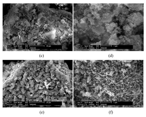
Fig. 3: Micrographs for the bi-metal co-precipitated catalysts at 2 magnifications: (a) Zn<sub>30</sub>Al<sub>40</sub> at 1000 times, (b) Cu<sub>60</sub>Al<sub>40</sub> at 15000 times, (c) Zn<sub>60</sub>Al<sub>40</sub> at 1000 times, (d) Zn<sub>60</sub>Al<sub>40</sub> at 15000 times, (e) V<sub>60</sub>Al<sub>40</sub> at 1000 times and (f) V<sub>60</sub>Al<sub>40</sub> at 15000 times.
