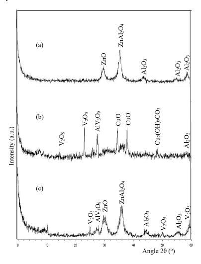
Fig. 4: XRD diffractograms of the catalyst samples (a)  $Cu_{30}Zn_{30}Al_{40}$  oxides, (b)  $Cu_{30}V_{30}Al_{40}$  oxides and (c)  $Zn_{30}V_{30}Al_{40}$  oxides.
