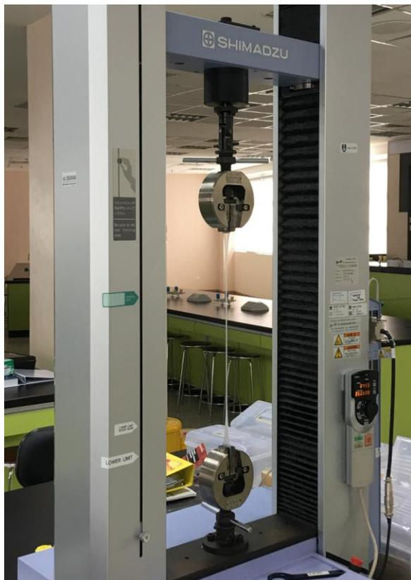
Fig. 1: Tensile test in progress
