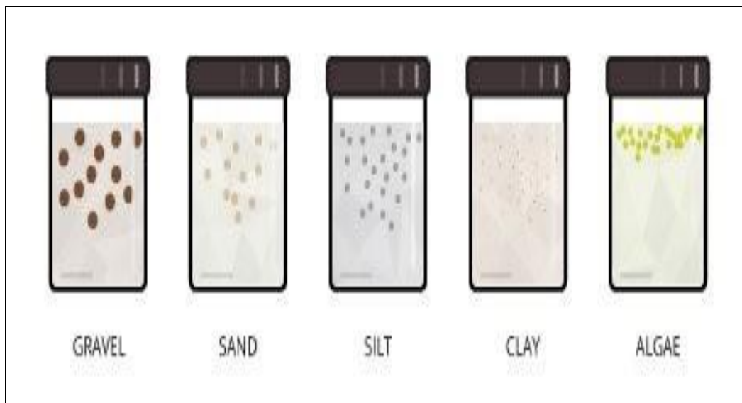
Figure 2.2 Both organic and inorganic particles of all size that contribute to the suspended solid concentration
