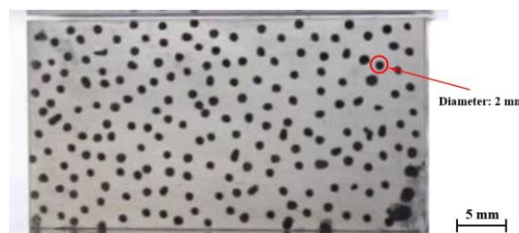
Figure 2. The front view of aluminium rectangular hollow tube with dots.
