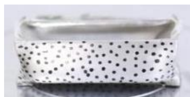
Figure 9. The damaged the aluminium rectangular tube.
