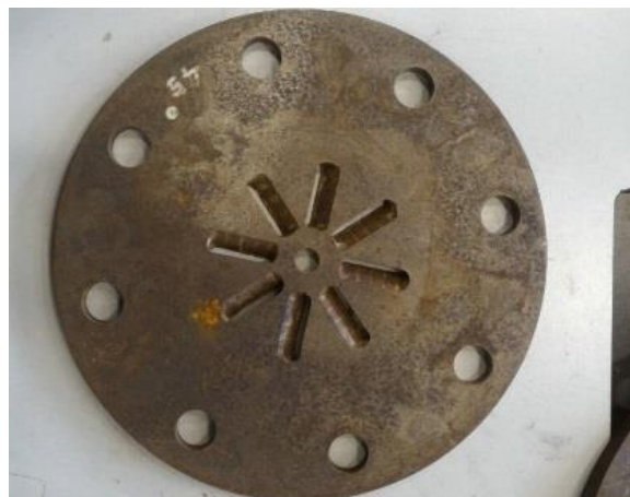
Figure 4. The 45° distributor that used in the fluidized bed dryer.
