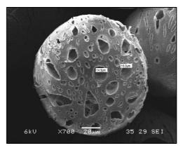
Fig. 1 SEM image of porous PCL microcarrier at 20% (w/v) camphene
