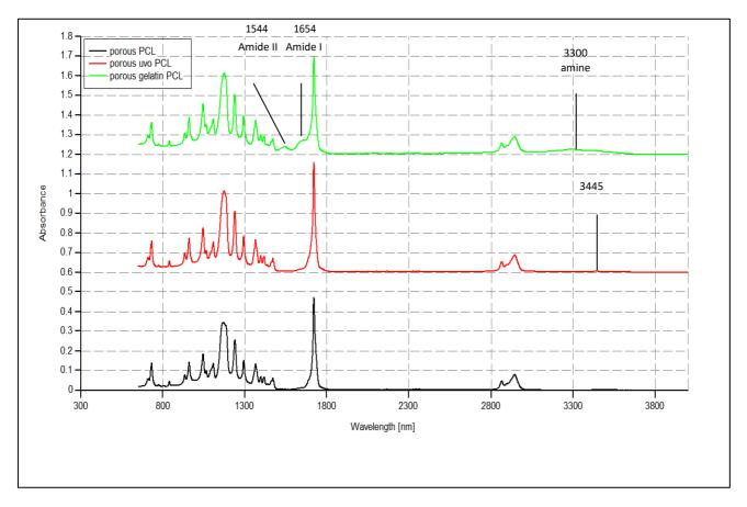
Fig. 2 ATR-FTIR spectra shows the elements content of the untreated PCL (porous PCL), UV/O<sub>3</sub> treated PCL (porous uvo PCL) and gelatin immobilized porous PCL (porous gelatin PCL).
