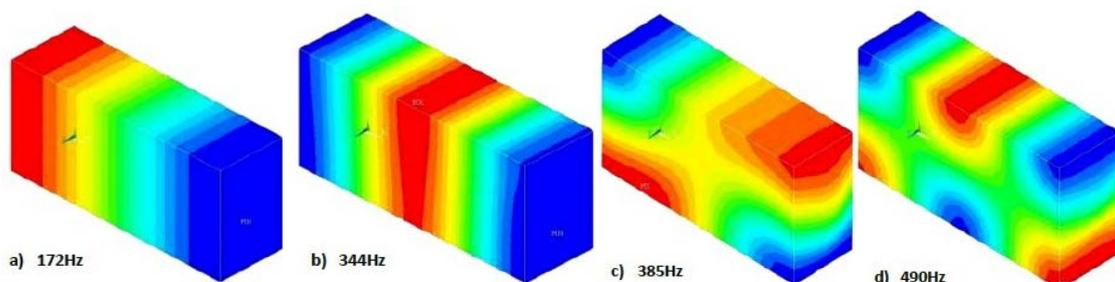
**Figure 3.** Mode shape of enclosure with a flexible wall
