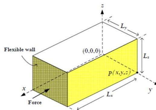
**Figure1.** Schematic diagram of rigid walled enclosure with a flexible wall
