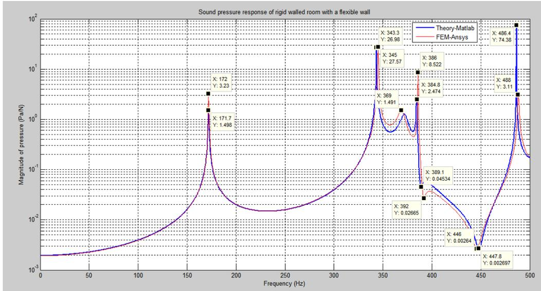
**Figure 2.** Magnitude of sound pressure response in a rigid walled cavity with flexible wall
