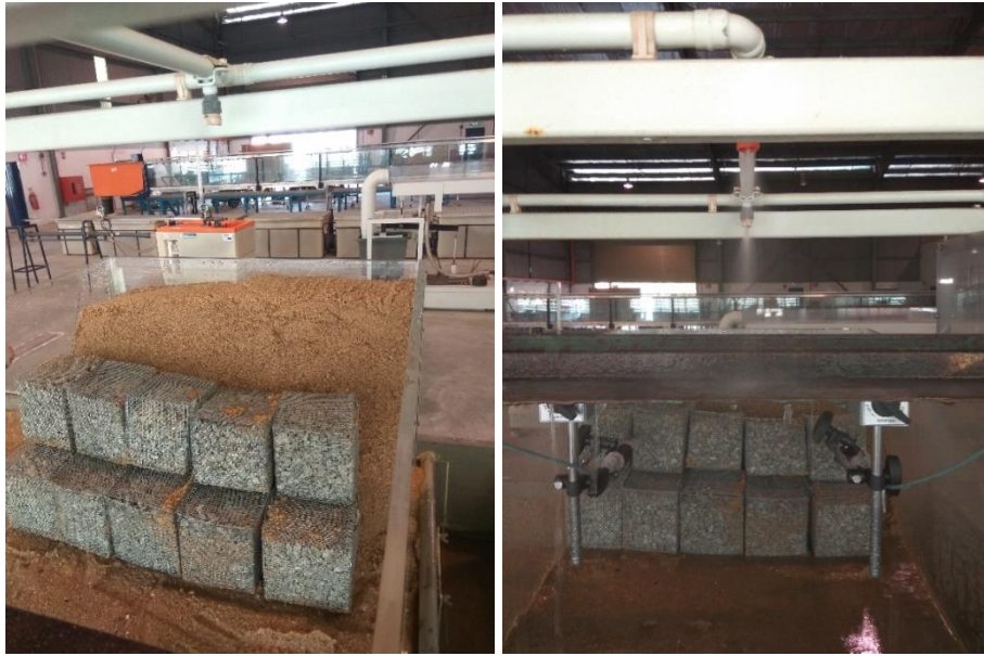
Figure 4.12 Gabion wall settled after exposed to the rainfall
