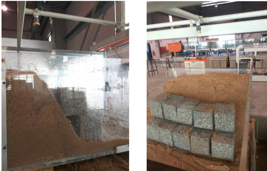
Figure 3.5 Arrangement of gabion wall at slope model
