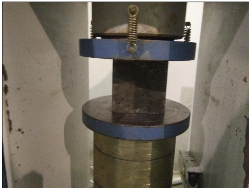
Figure 3.19 Compressive strength test in progress
