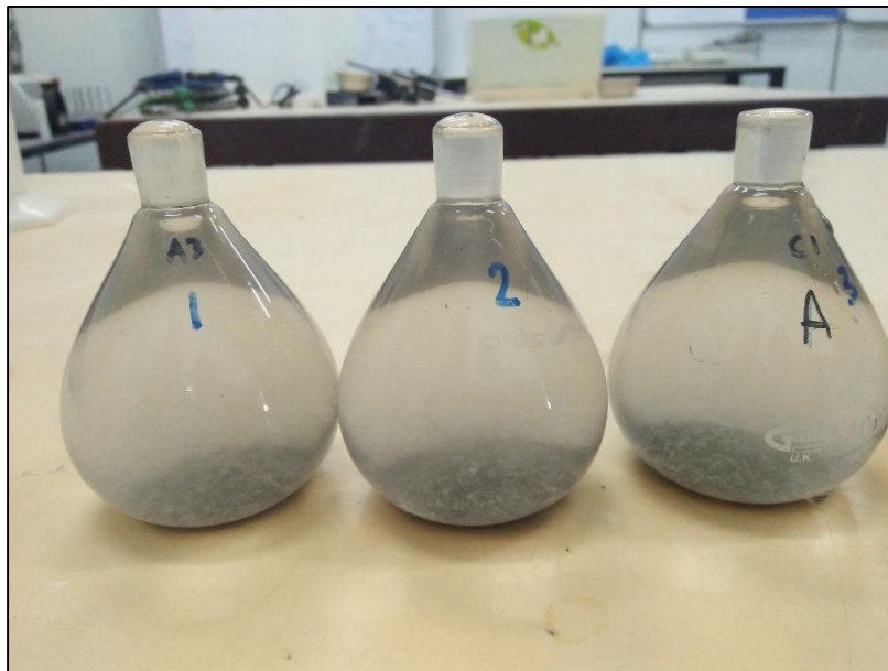
Figure 3.11 Pycnometer test of CBA
