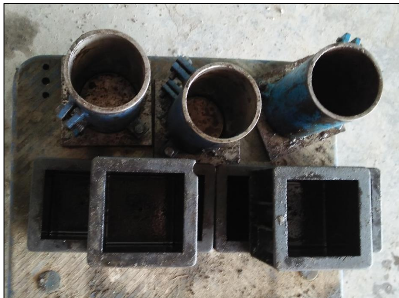
Figure 3.16 Cube and cylindrical mould used in research
