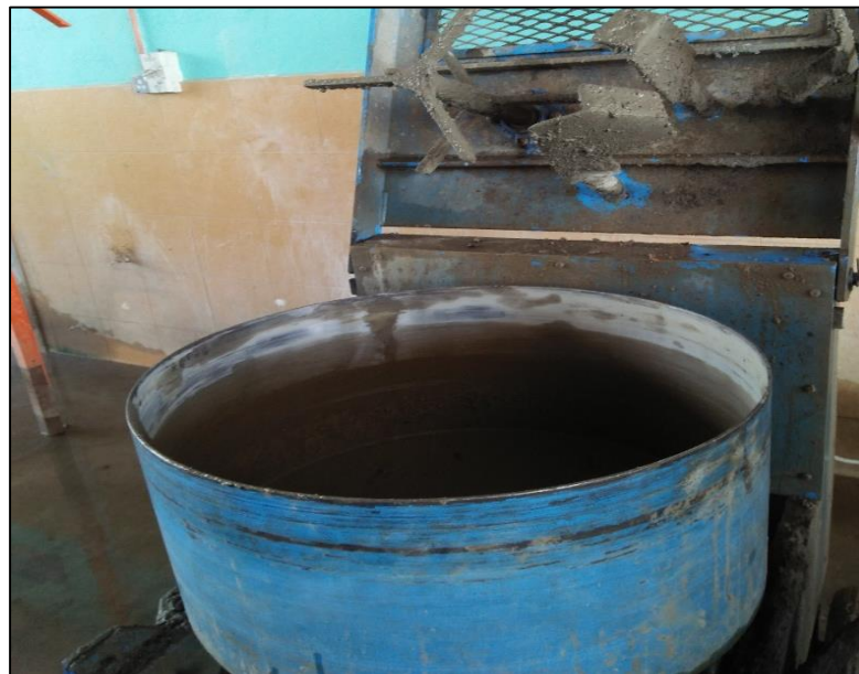
Figure 3.14 Mixer machine used in concrete batching
