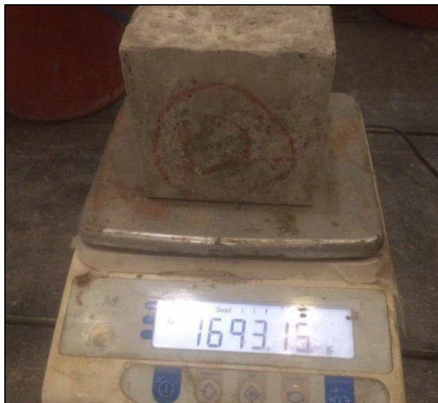
Figure 3.18 Weighing concrete specimen
