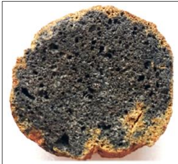
Figure 2.6 Pores structure of lightweight aggregate concrete Source: Ayati (2018).
