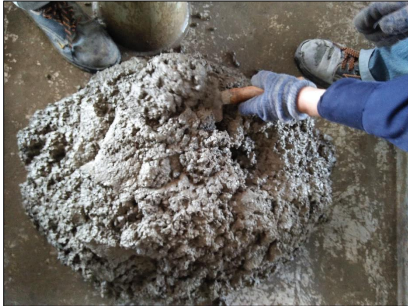
Figure 3.15 Concrete after being mixing in mixer machine
