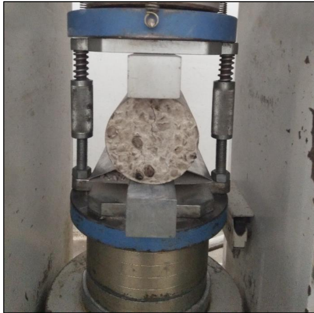
Figure 3.20 Splitting tensile strength test in progress
