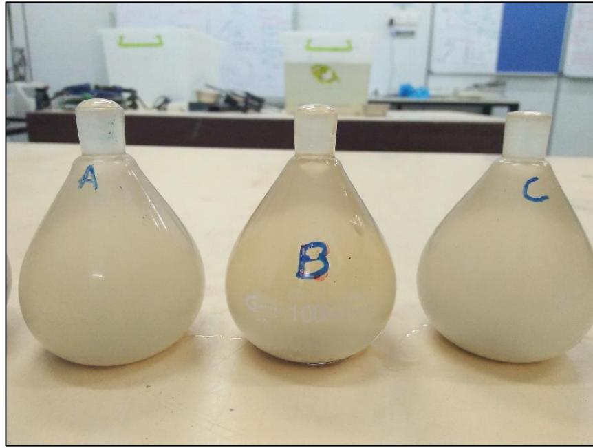
Figure 3.8 Pycnometer test of sand
