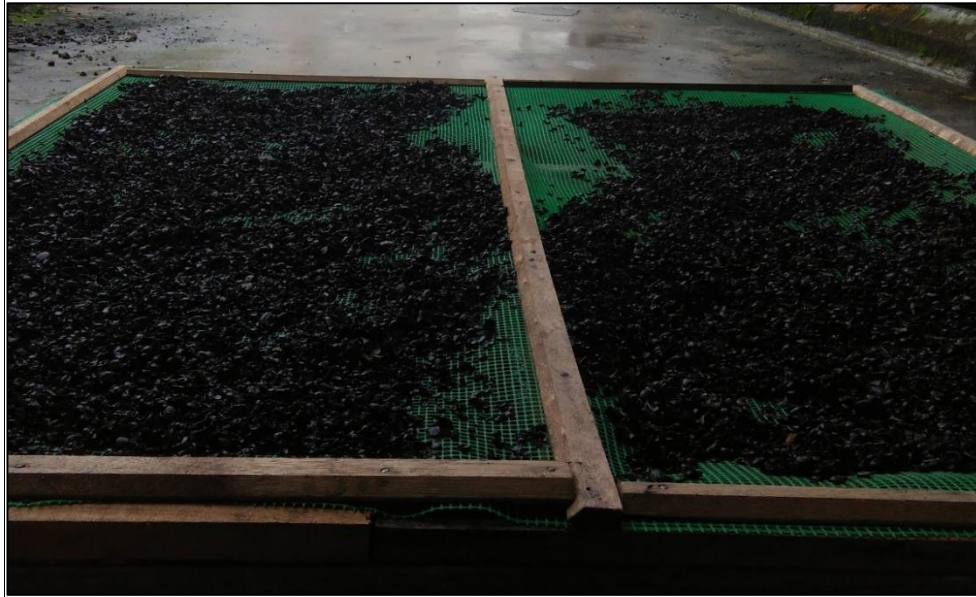
Figure 3.5 OPS was put on net to remove excessive water
