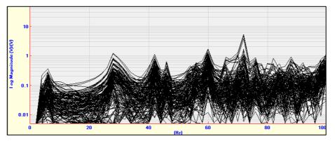
Figure 8. Response sample of roving hammer impact hammer test with three accelerometers.
