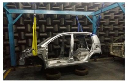
Figure 4. Hanged BIW structure under test rig in a free-free boundary condition.
