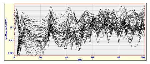
Figure 6. Response sample of roving hammer impact hammer test with one accelerometer.
