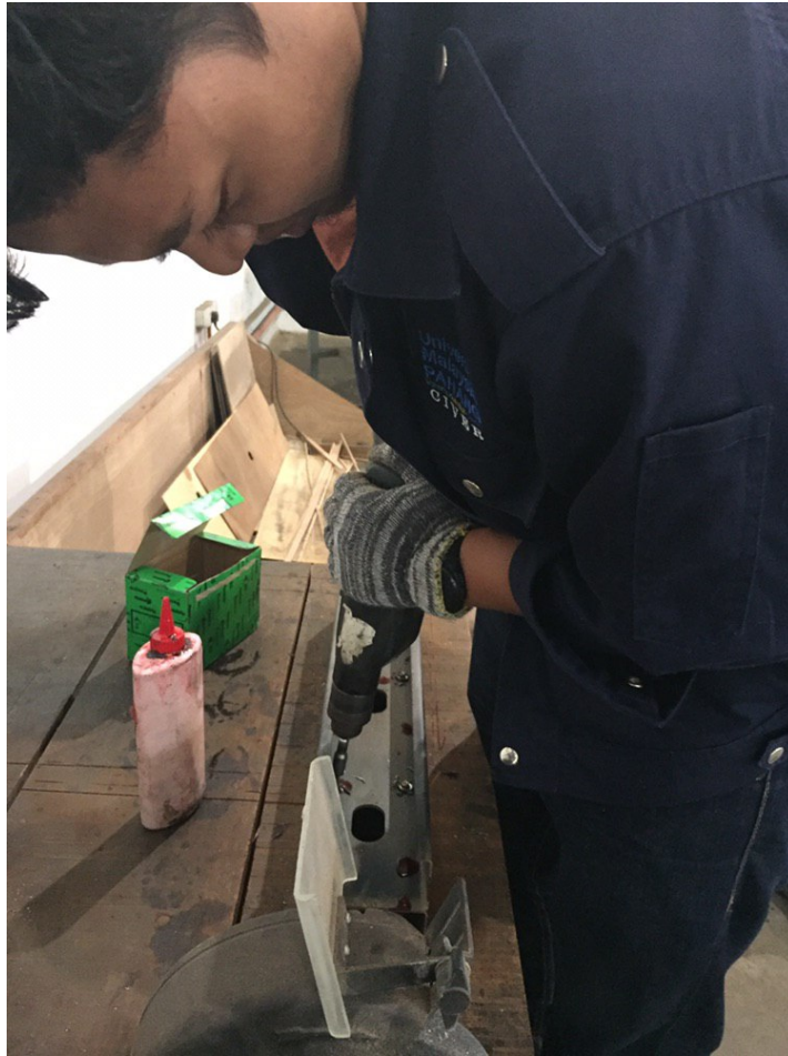
Figure 3. 5: Drilling of specimens
