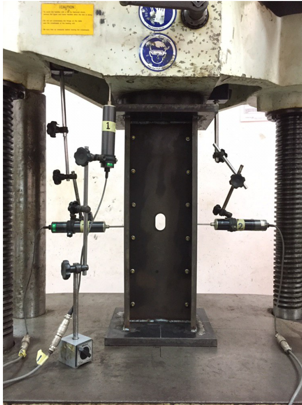
Figure 3. 3: Positioning of specimens and transducers in Universal Testing Machine
