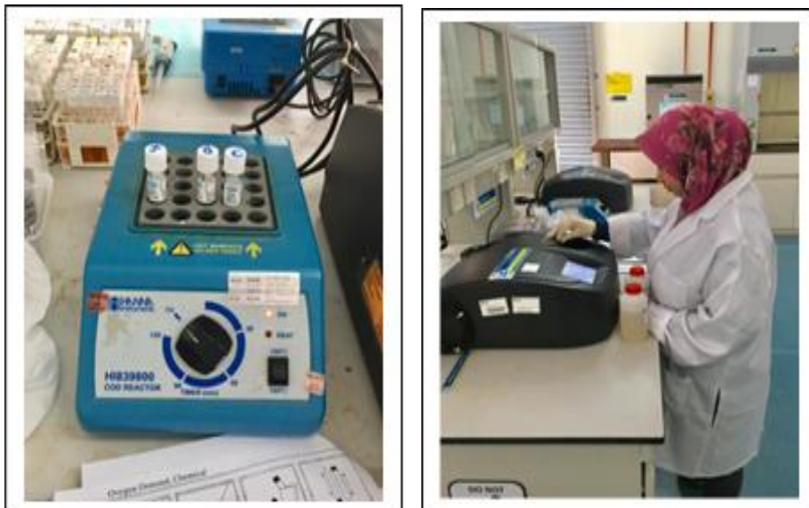
Figure 3.13 Chemical Oxygen Demand (COD) Experiment
