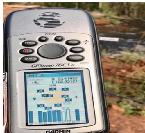
Figure 3.6 Determining position of sampling station
