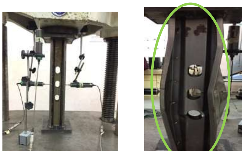
Figure 4.5 Buckling behaviour for BE103-1.2-A3
