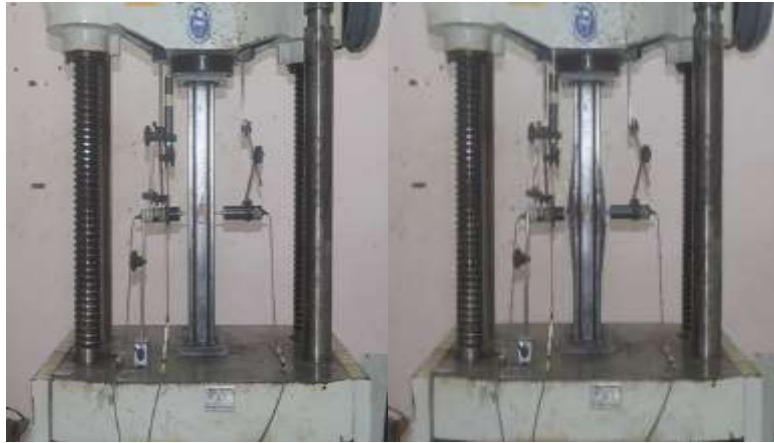
Figure 4.9 Bucking behaviour for BE103-2.0-A2
