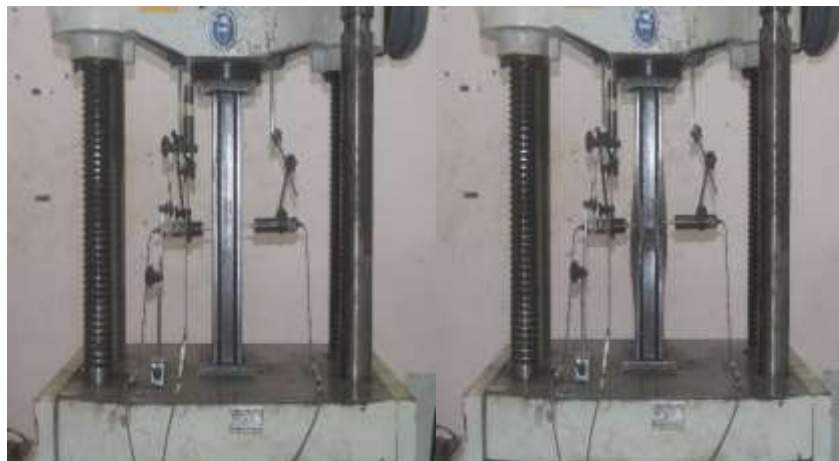
Figure 4.8 Bucking behaviour for BE103-2.0-A1
