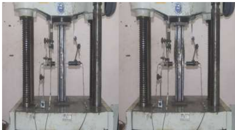
Figure 4.10 Bucking behaviour for BE103-2.0-A3
