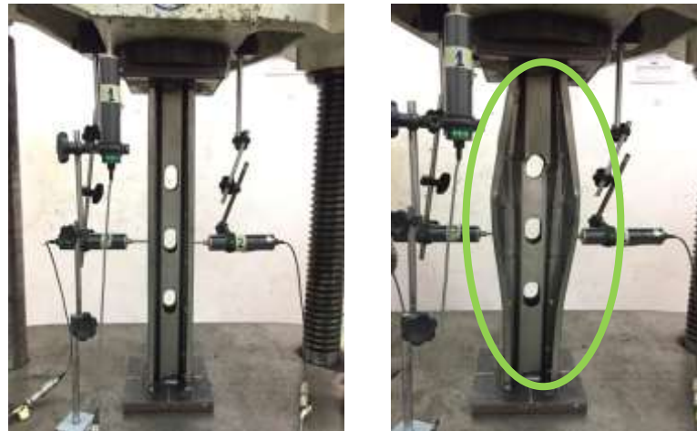
Figure 4.6 Buckling behaviour for BE103-1.2-A4
