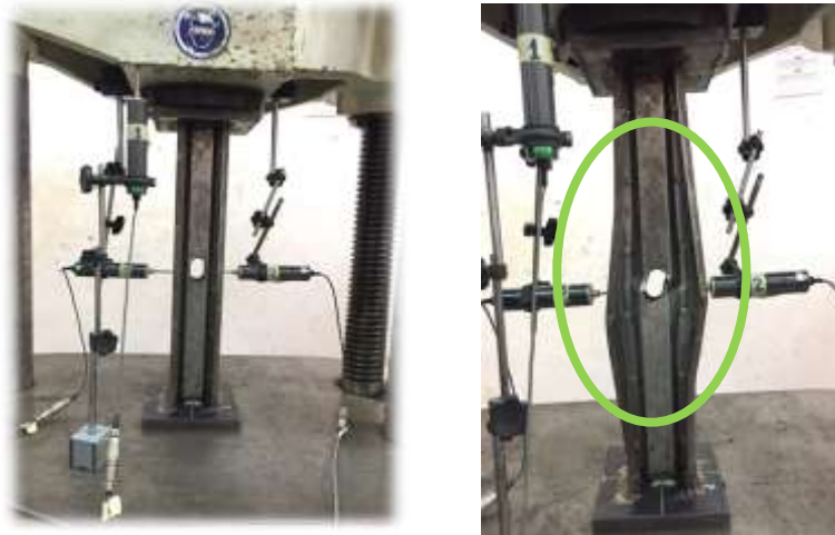
Figure 4.4 Buckling behaviour for BE 103-1.2-A2
