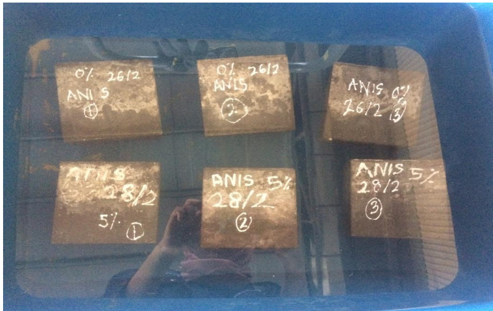
Figure 3.6 Water Absorption Test
