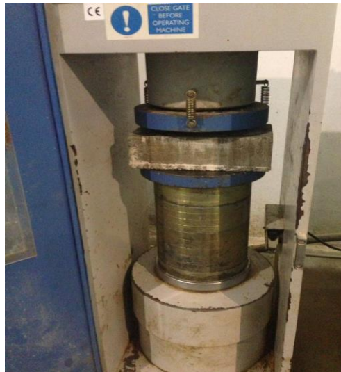
Figure 4.2 Compressive strength test for 0% replacement
