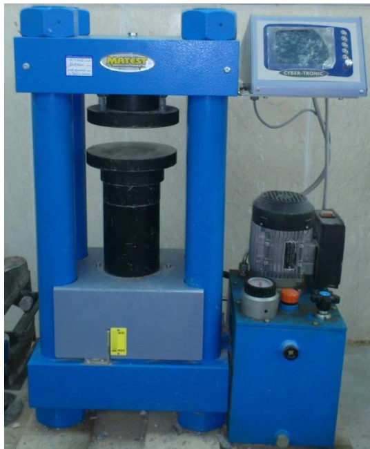
Figure 2.4 Compressive strength machine
