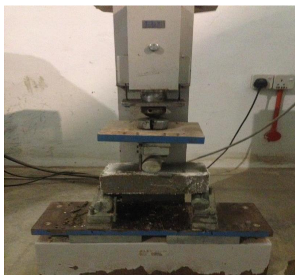
Figure 4.5 Flexural strength test for 0% replacement
