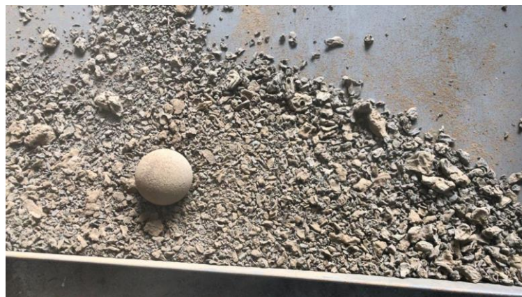
Figure 3.7 Dry sludge after grind before sieve
