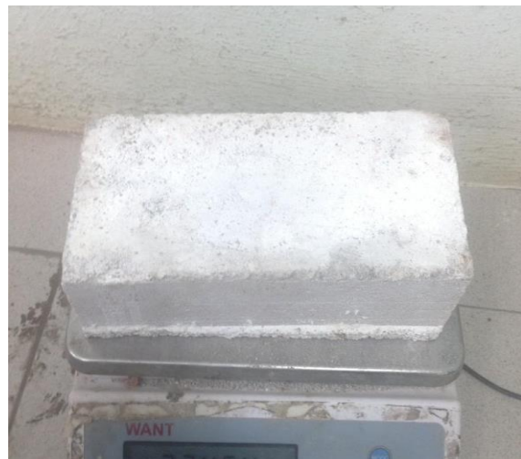
Figure 4.9 Specimen weighed after water absorption test
