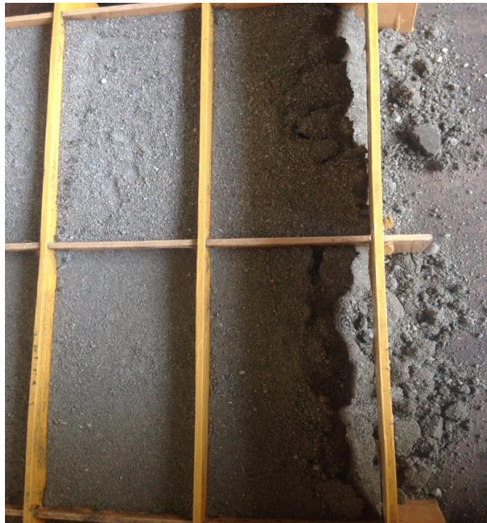
Figure 4.10 Condition of sand brick with 5% replacement after casting process
