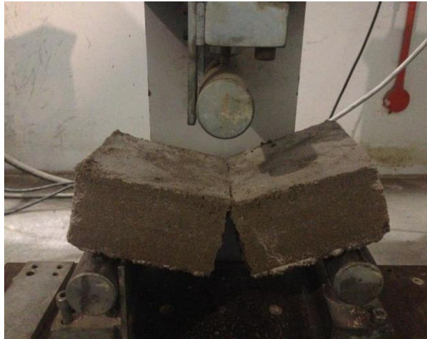
Figure 4.6 Specimen of 0% replacement after flexural strength test
