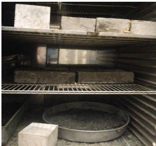
Figure 4.8 Specimens dried in the oven before water absorption test
