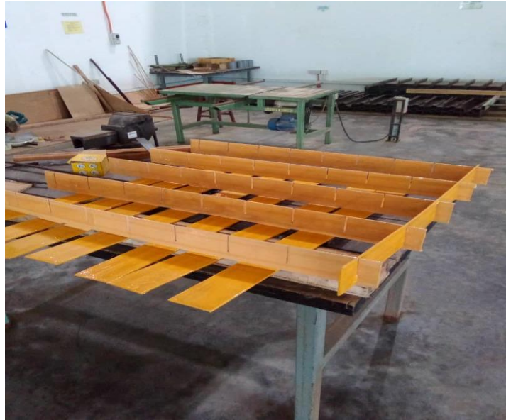
Figure 3.9 Preparation for the brick mould
