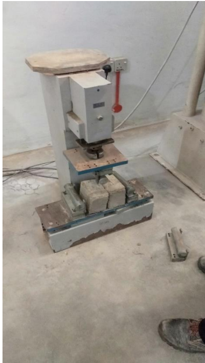
Figure 3.12 Machine Flexural Strength
