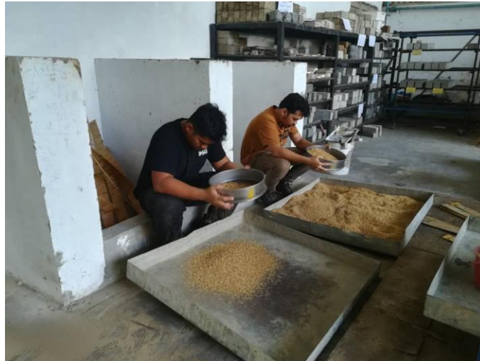
Figure 3.6 Process Sieve Rice Husk from Other Materials
