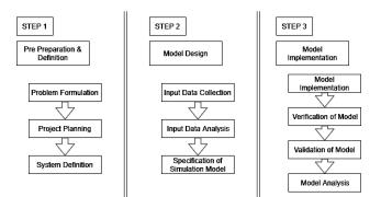
Figure 3 Model building procedure for production simulation
