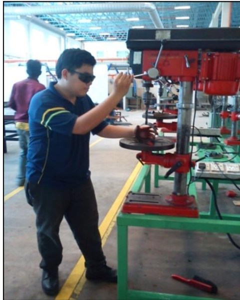
Figure 3.10: Drilling using drill press.
