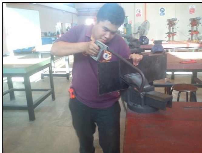
Figure 3.7: Cutting sheet metal using hand saw.
