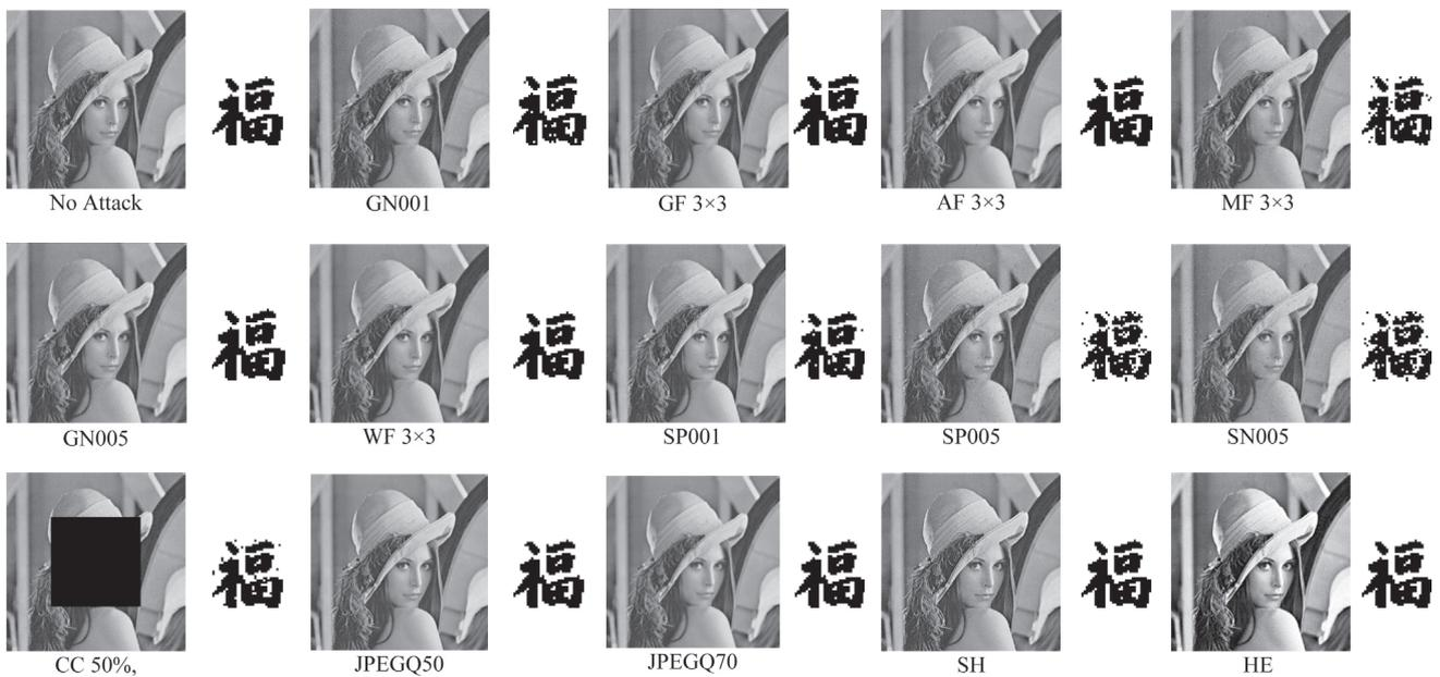
Fig. 9. Watermark recovery from various attack.
