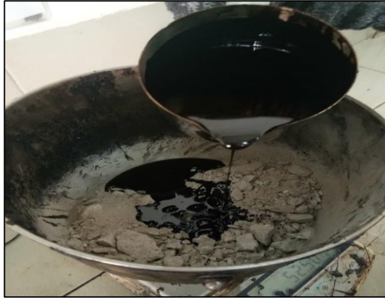
Figure 3.5 Bituminous content with 4.5% by weight of aggregate
