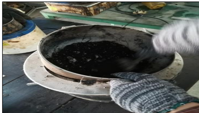
Figure 3.8 Mixing sample at temperature 150 between 155°C.
