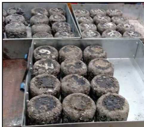
Figure 3.43 Condition of sample after Cantabro Loss testing
