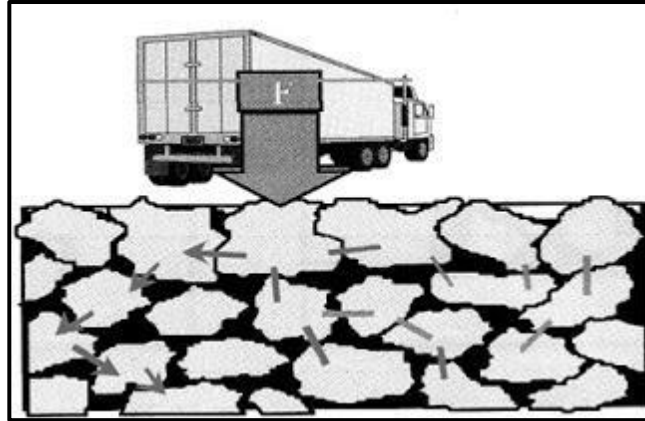
Figure 2.4 The stability in a SMA-m ix is obtained through the internal friction in the self -supporting stone skeleton
