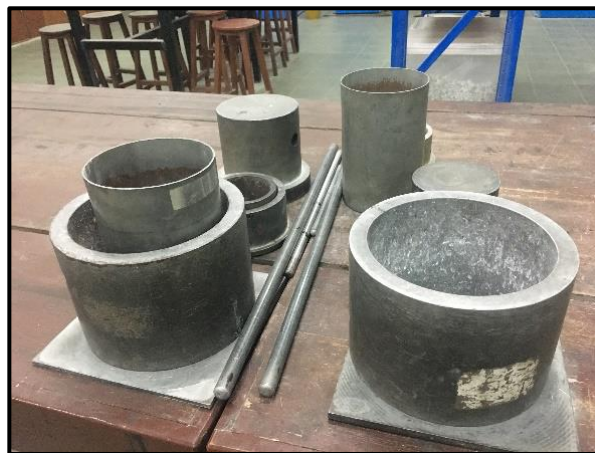
Figure 3.13 Open ended steel cylinder with plunger and base plate, tamping rods and the cylindrical metal measures.
