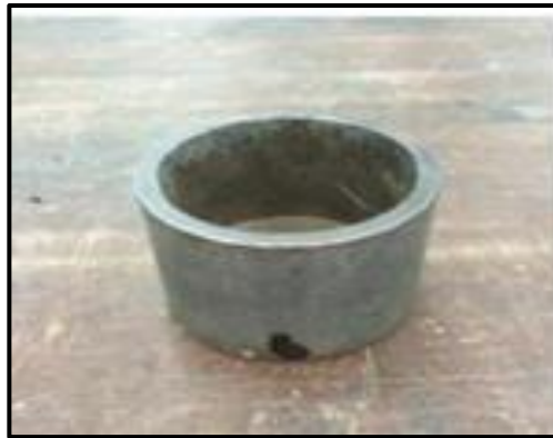
Figure 3.8 A cylinder of internal for measuring aggregate
