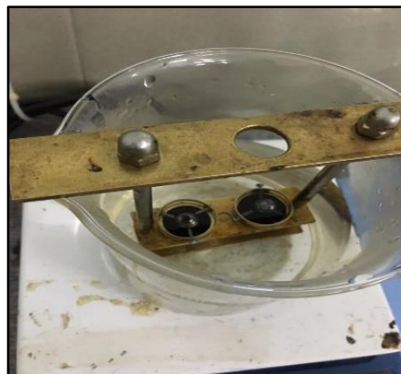
Figure 3.28 Steel balls is being placed on the surface of the bitumen in the ring
