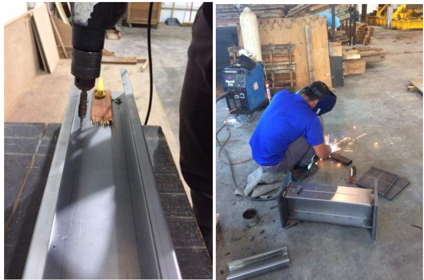
Figure 2.6 Screws and welding at the specimen.
