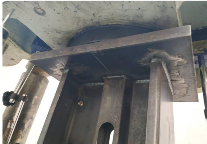
Figure 3.7 Support at the above of specimen.
