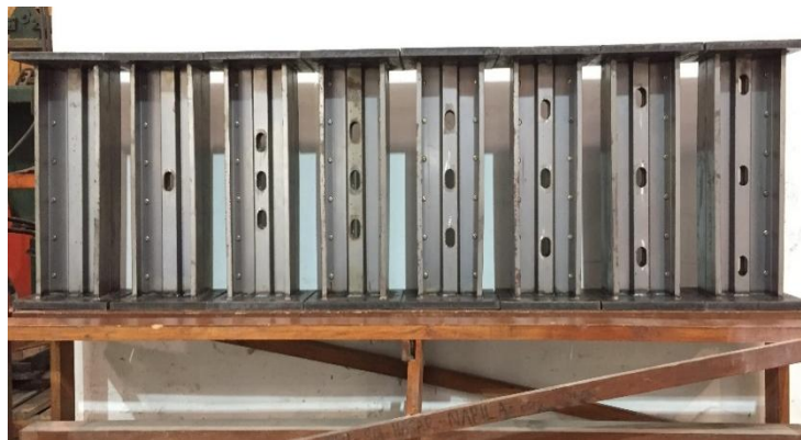
Figure 3.5 Series of Cold-Formed E section
