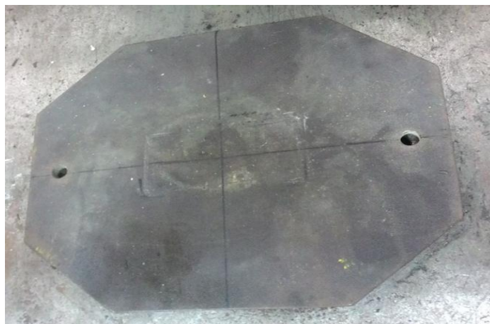
Figure 3.9 Bearing plate at the bottom.
