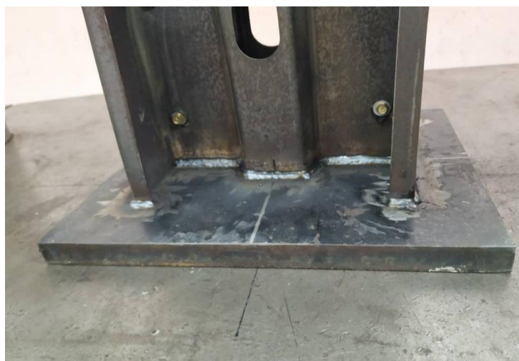
Figure 3.6 Support at the bottom of specimen.
