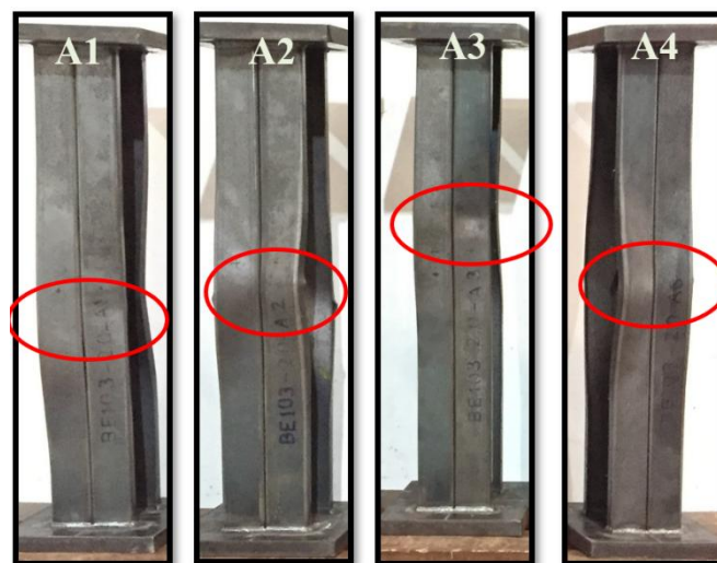
Figure 4.4 Side view failure mode BE103-2.0
