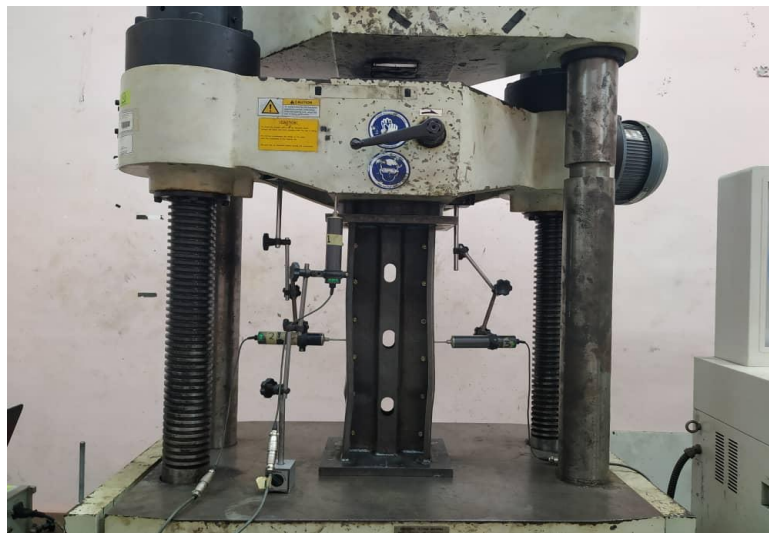
Figure 3.23 Universal testing machine and transducers set-up.
