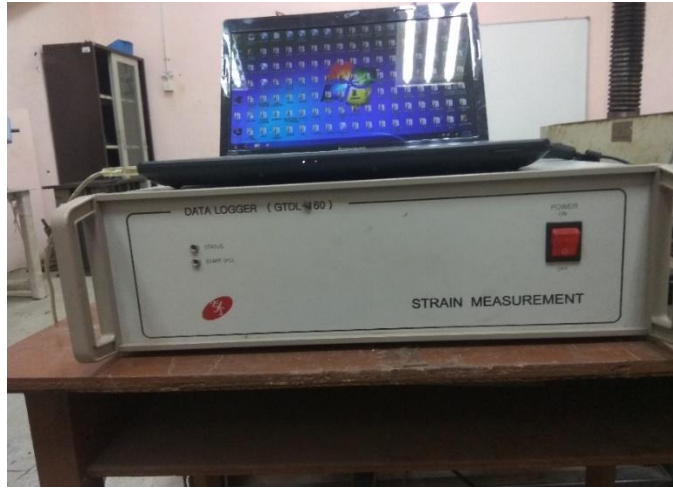
Figure 3.10 Data logger (Strain Measurement)
