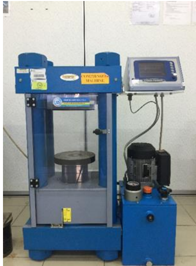
Figure 3. 11 Compression Testing Machine
