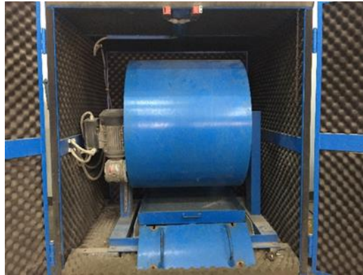
Figure 3. 12 Los Angeles Abrasion Machine
