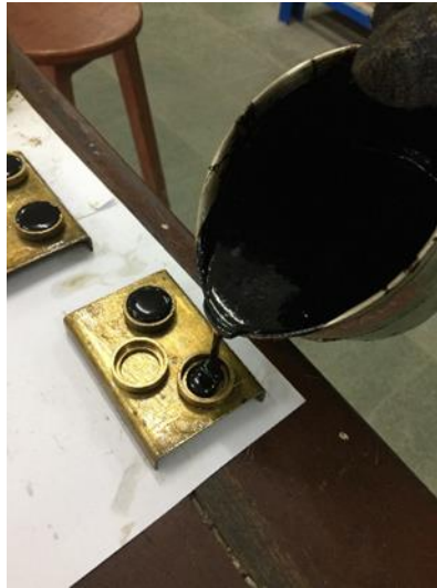
Figure 3. 3 Bitumen poured in the brass rings
