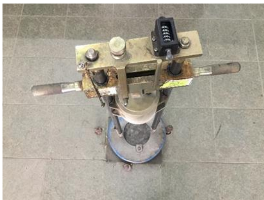
Figure 3. 10 Anggregate Impact Testing Machine
