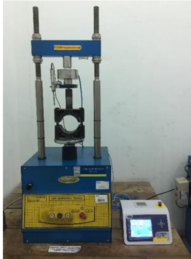
Figure 3. 13 Marshall Compression Machine
