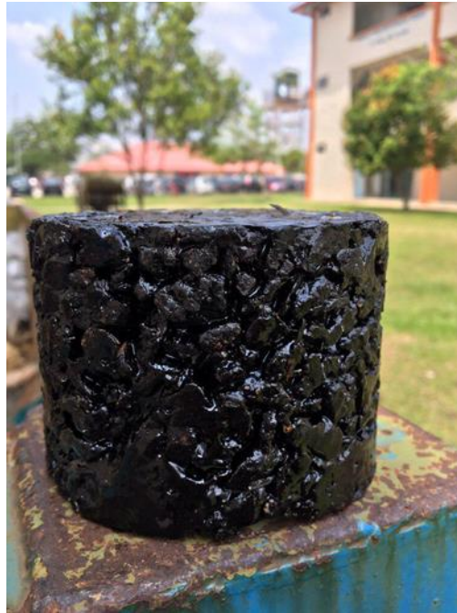
Figure 2. 4 Stone Mastic Asphalt
