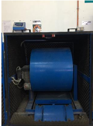
Figure 3. 14 Los Angeles Abrasion Machine Testing
