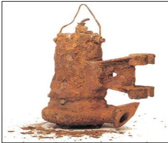
Figure 2.3 Uniform Corrosion on Competitor's cast iron pump
