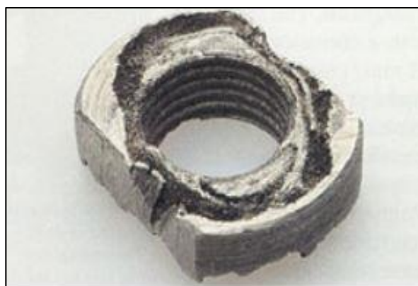
Figure 2.5 Crevice corrosion on stainless steel nut exposed to seawater
