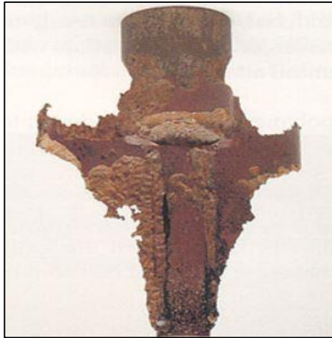
Figure 2.10 Erosion corrosion on impeller
