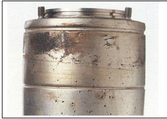
Figure 2.4 Pitting corrosion on stainless steel stator housing operating in seawater
