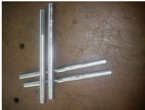
Figure 3.27: Mild steel shaft with diameter 12mm
