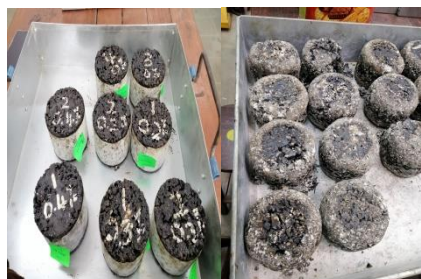
Figure 3.12 Samples of porous asphalt before and after the test
