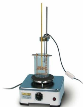
Figure 3.8 Apparatus of Softening point of bitumen
