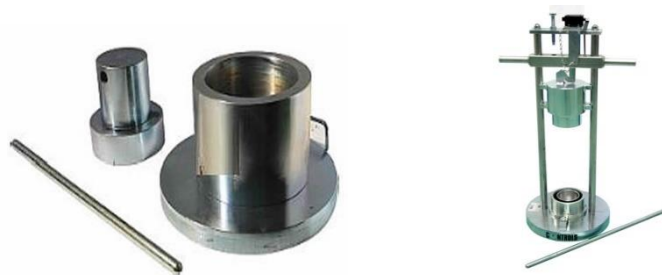
Figure 3.6 Open ended steel cylinder with plunger, tamping rod and compression testing machine
