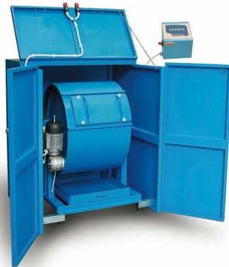
Figure 3.11 Los Angeles Abrasion Machine without steel balls
