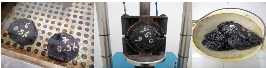
Figure 3.13 Sample of Porous Asphalt
