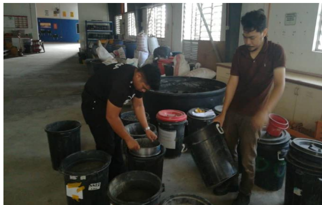
Figure 3.8 Sieve palm oil clinker passing 4.75 mm
