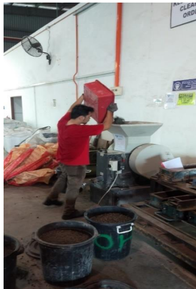
Figure 3.7 Crushing the large palm oil clinker
