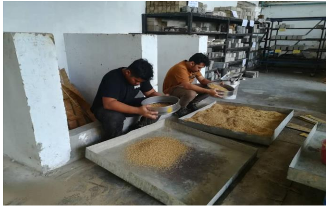
Figure 3.9 Sieve rice husk to get passing 4.75 mm
