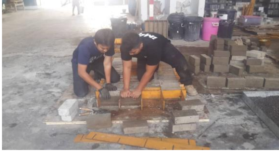
Figure 3.11 Demoulded the brick from the formwork
