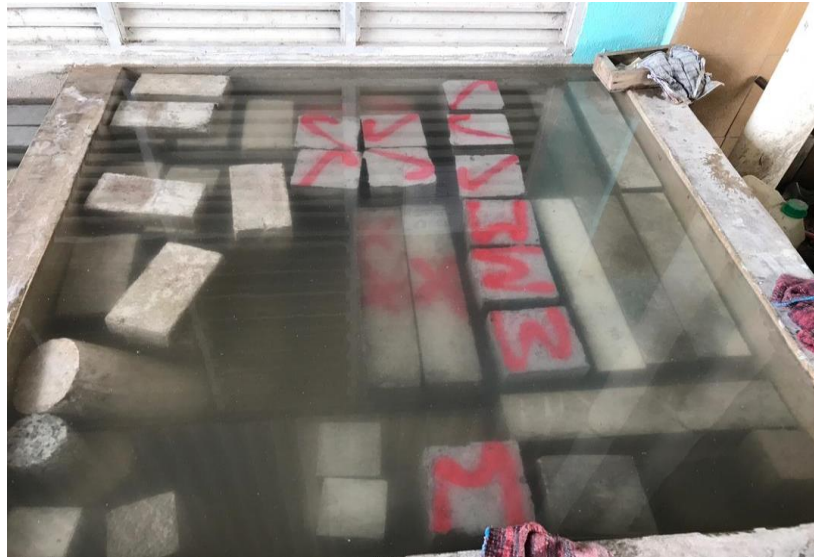
Figure 3. 7: concrete during water curing
