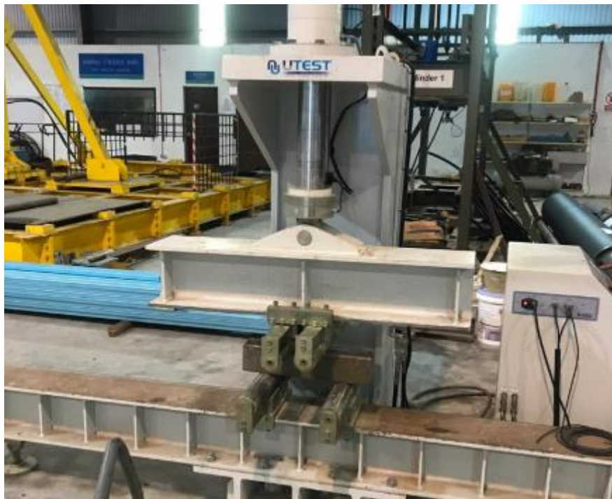
Figure 3. 10: Beam under flexural strength machine
