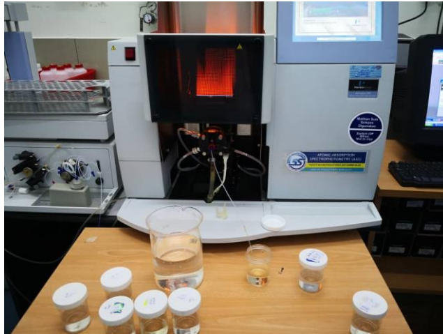
Figure 3.4: Analysis using AAS (Atomic Absorption Spectroscopy)
