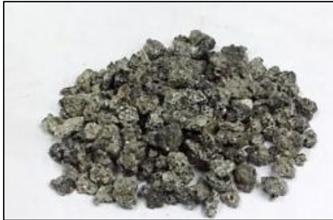
Figure 3. 7 Palm oil clinker with nominal size 5 mm
