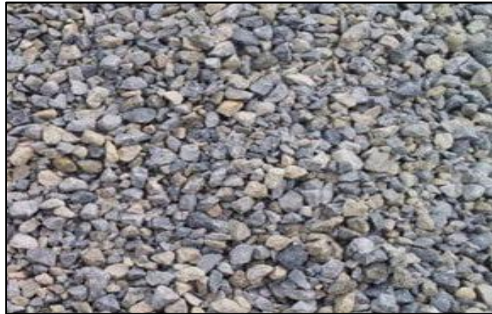
Figure 3. 3 Natural Crushed Gravel with nominal size of 5mm
