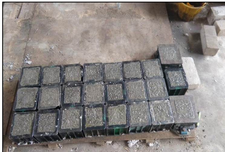
Figure 3. 10 Cubic mould was stored in dry area for 24 hours after casting
