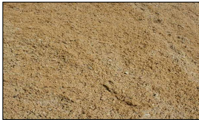
Figure 3. 5 Natural river sand with nominal size of 300 \mu\text{m}
