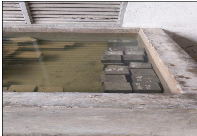
Figure 3. 12 Specimens were cured in water curing
