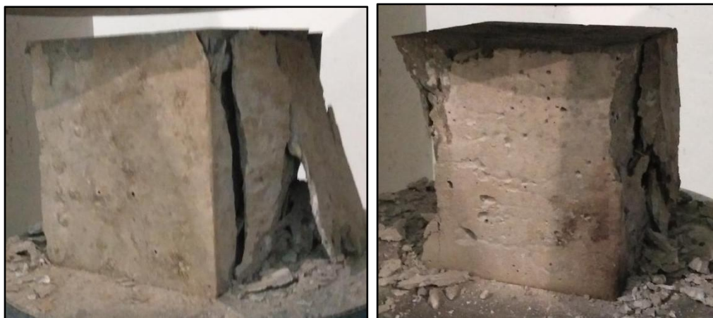
Figure 4. 9 Failure mode of POC-UHPC cubic specimen
