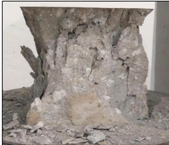
Figure 4. 8 Failure mode of plain UHPC cubic specimen
