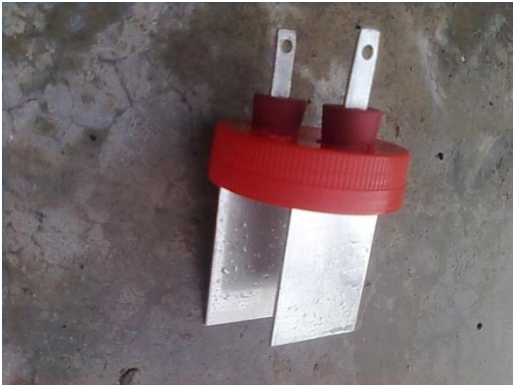
Figure 3.16 Joining plate and cork
