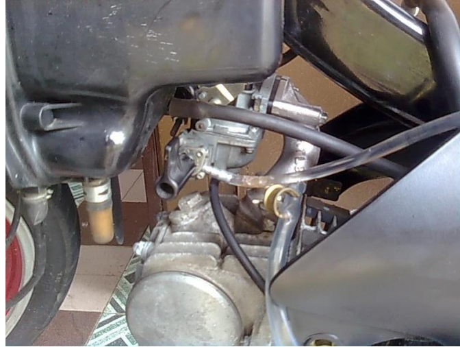
Figure 3.19 connection tubes fuel and hydrogen gas to carburetor.
