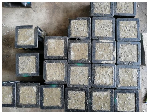
Figure 3.10 Plastic mould was stored in room temperature for 24 hour
