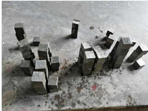
Figure 3.11 UHPC specimens for compressive strength test
