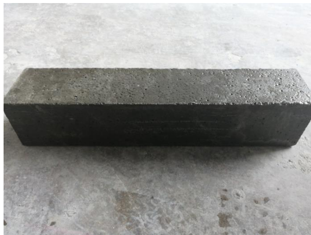
Figure 3.12 UHPC specimens for flexural strength test
