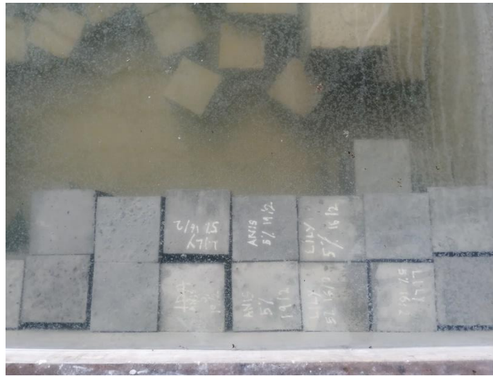
Figure 3.13 The specimens cured in water tank
