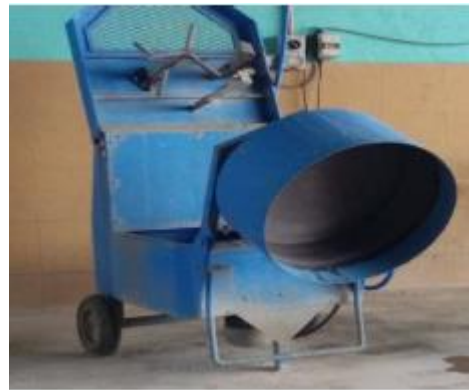
Figure 3.9 Concrete pan mixer used for mixing process
