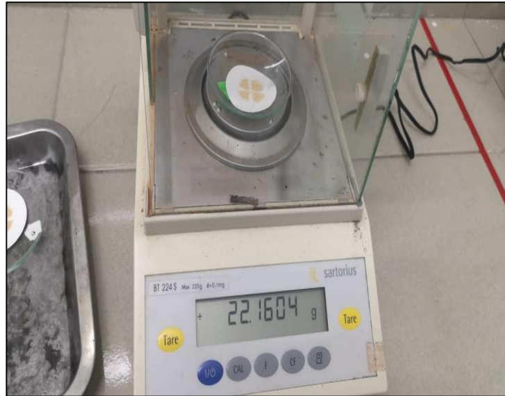
Figure 3.10 Result of weight of filter paper by using Balance GR200
