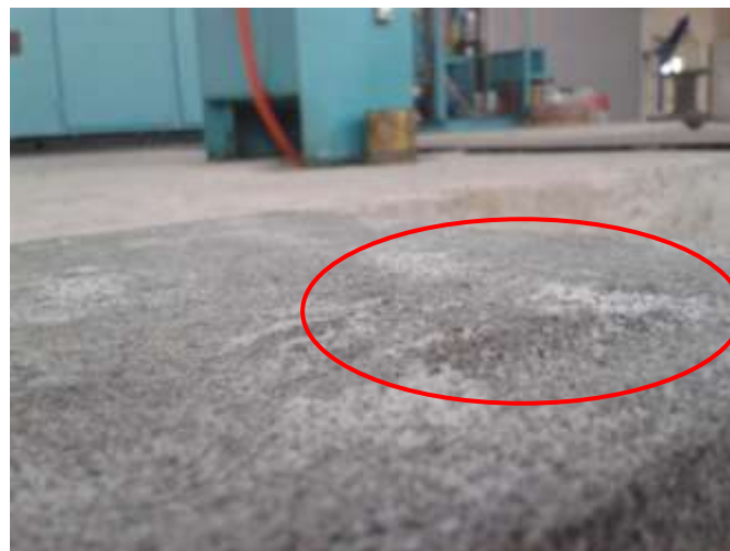
Figure 4.16: Drop Defect. It has contour on flat surface.
