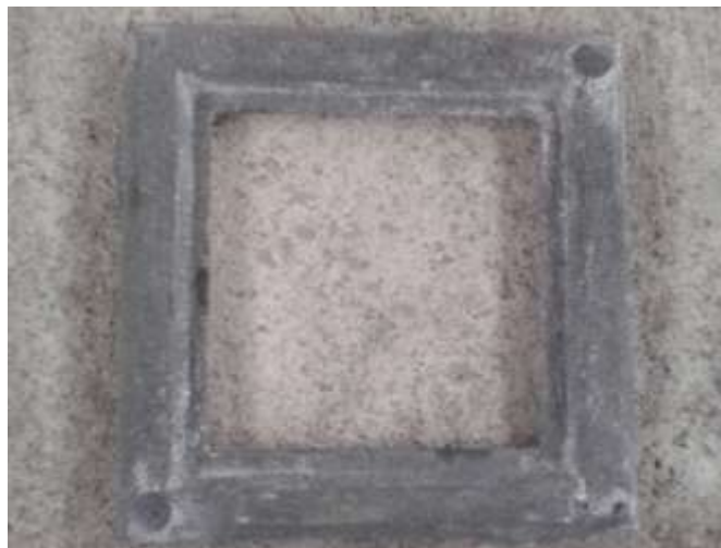
Figure 4.8: The frame without the sprue and riser, top view.
