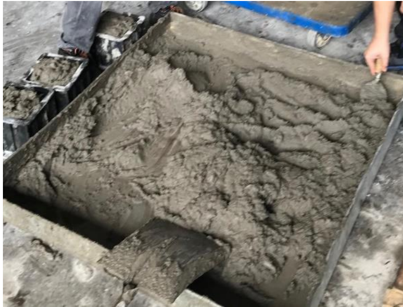
Figure 3.9 Fresh Foamed Concrete
