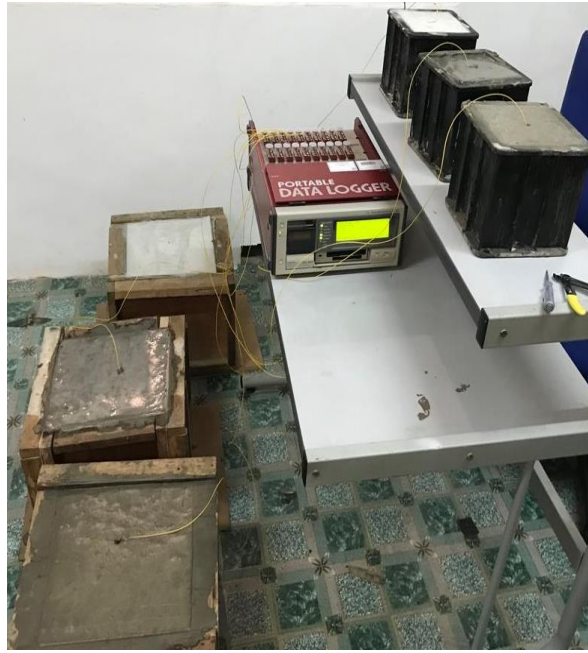
Figure 3.14 Heat of Hydration Setup
