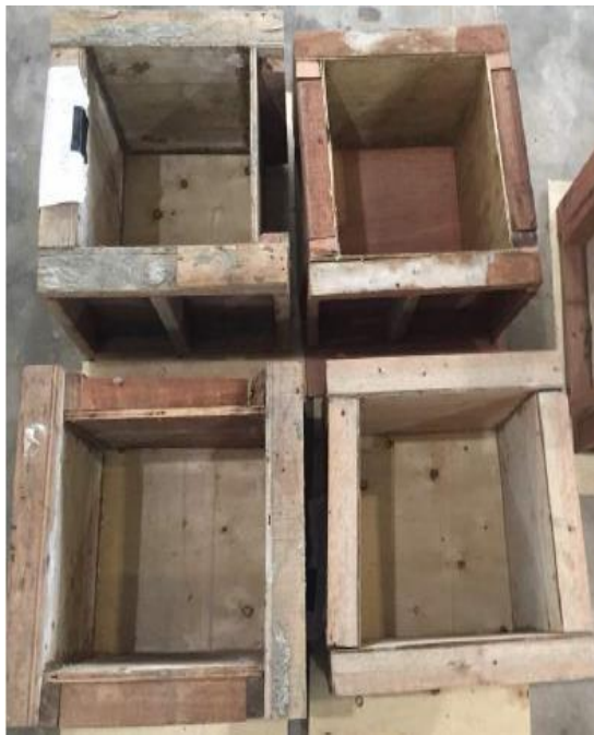
Figure 3.13 Prepartion of Specimens of Heat of Hydration
